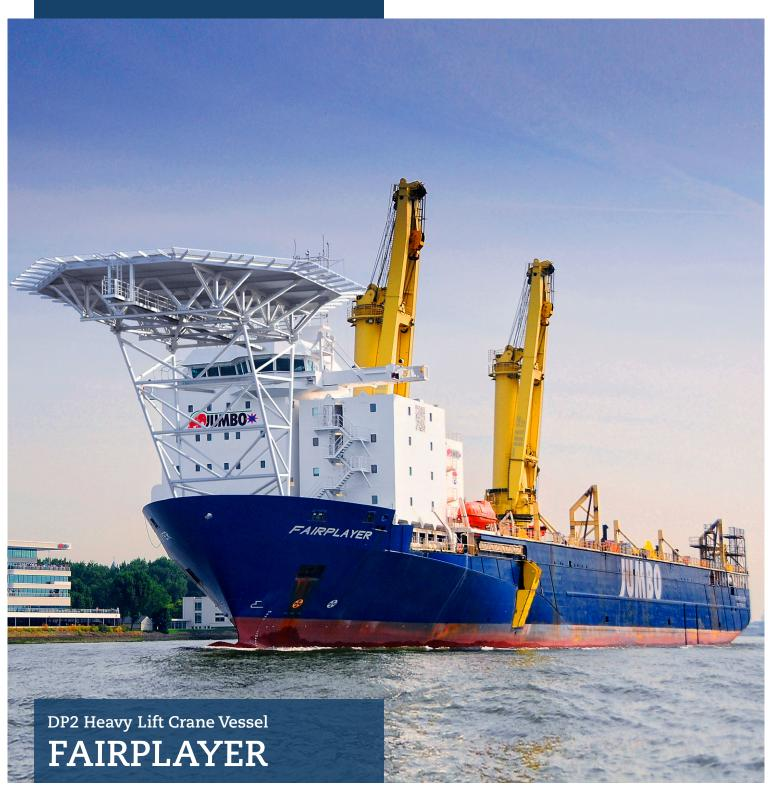
A multi-functional dynamic positioned Heavy Lift Crane Vessel (HLCV) suited to the offshore requirements of the Energy Industry worldwide.
